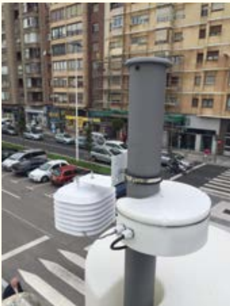
NO 2 and O 3 sensors deployed in the city of Santander, Spain
