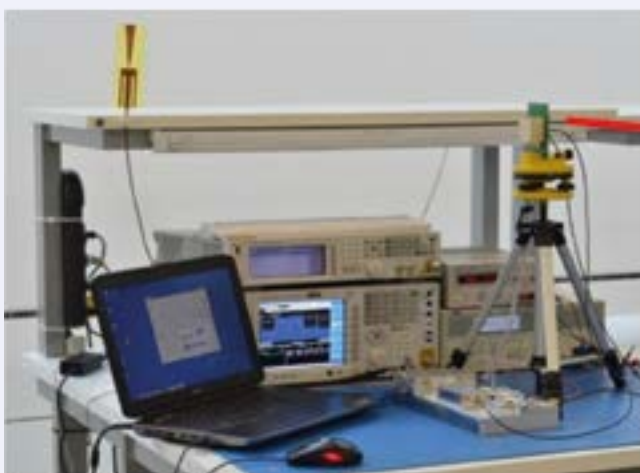
Figure 1: Carrier aggregation demonstrator setup comprising the reconfigurable RF front-end (including a dual band miniature antenna), the control PC and the measurement equipment
